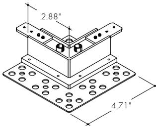
For creating a 90° in-plane corner. For use with FF Front Flange and STJOIN-EF Electrical Joiner only.
